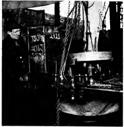
A scarphing machine designed at the Skinner & Eddy yard in Seattle and now extensively used in the Northwest.
